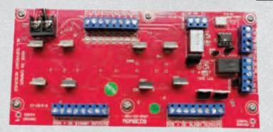
The MOM8ECB provides power across independently protected channels which will switch on or off with the Fire Alarm Control Panel input. These are distribution boards used for Access Control Systems and Egress Doors. Power can be transferred in the event of an alarm from the primary set of 8 channels to a secondary set of 8 channels, allowing the ability to drop power to magnetic doors locks while engaging electric strikes.
