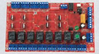
The ACM4ECB and ACM8ECB are used with an access control system to power Egress doors and to isolate the access control system from coil induced voltage spikes. Each powered relay output is triggered by an independent input. The ACM also provides Fire Alarm Control Panel (FACP) activation with either latching or non-latching functionality to drop power to selected Egress doors.
